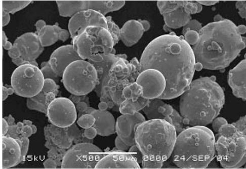
**Fig. 6.** SEM micrograph of Fe-Co powder particles used in this study
